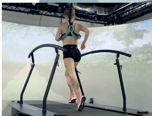
Patients use the quantitative gait analysis BeMoveD to measure forces and moments when walking. Movement patterns, muscle activity and joint load are analyzed with this method.
